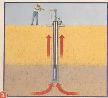
At the top of the well, install a pump powered by a motor or human effort to pull up water.
